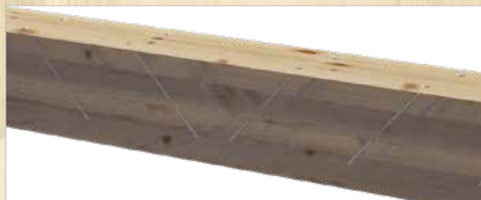
Reinforcement by coupling of beams
