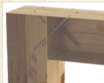
Joint between two girders
